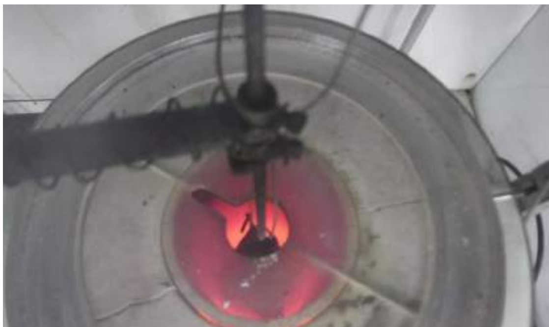
Photo No. 15 ASTM E136 Non-combustibility Test Setup with Specimen in Furnace
