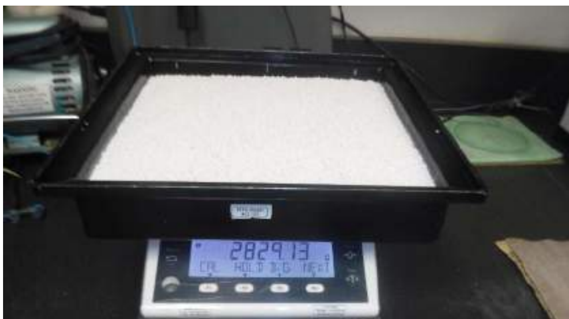
Photo No. 16 ASTM E96 Preparation of Desiccant and Pan
